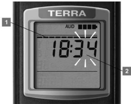
Figure 22 – LCD of the dosimeter (the submode of time and date correction – time programming)
