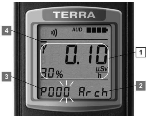
Figure 10 – LCD of the dosimeter (the submode of measurement result saving of photon-ionizing radiation DER)
