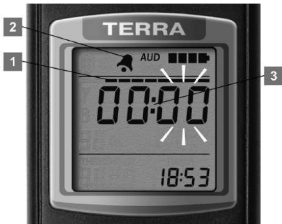
Figure 26 – LCD of the dosimeter (the submode of alarm clock activation time programming)
