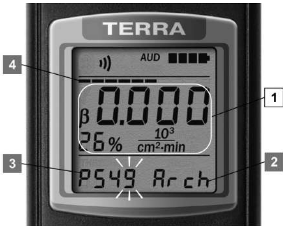
Figure 20 – LCD of the dosimeter (the submode of measurement result saving of surface beta-particles flux density)
