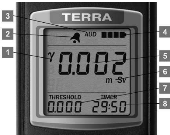
Figure 11 – LCD of the dosimeter (the mode of indication of photon-ionizing radiation DE accumulated value)
