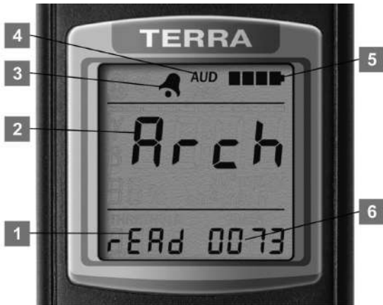
Figure 29 – LCD of the dosimeter (the mode of measurement results viewing stored in the nonvolatile memory)
