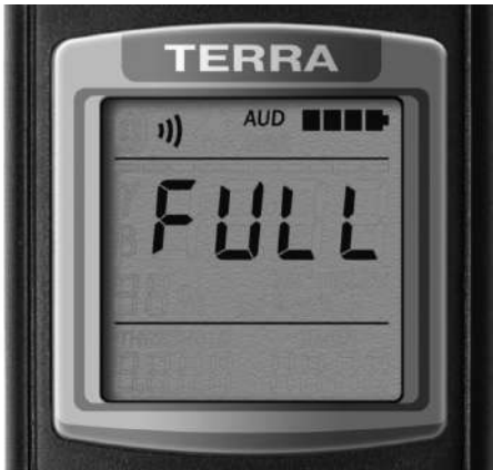
Figure 19 – LCD of the dosimeter (start of the submode of measurement result saving – no free space in the nonvolatile memory)
