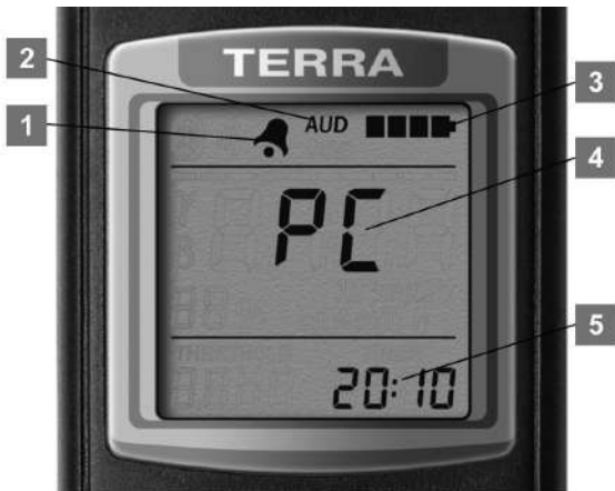
Figure 27 – LCD of the dosimeter (the mode of data communications control with the PC)
