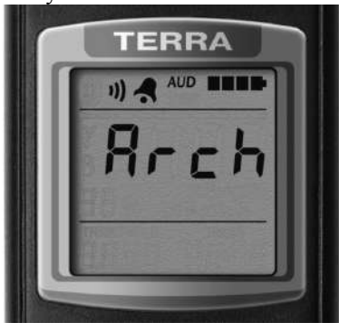
Figure 16 – LCD of the dosimeter (start of the submode of measurement result saving in the nonvolatile memory)
