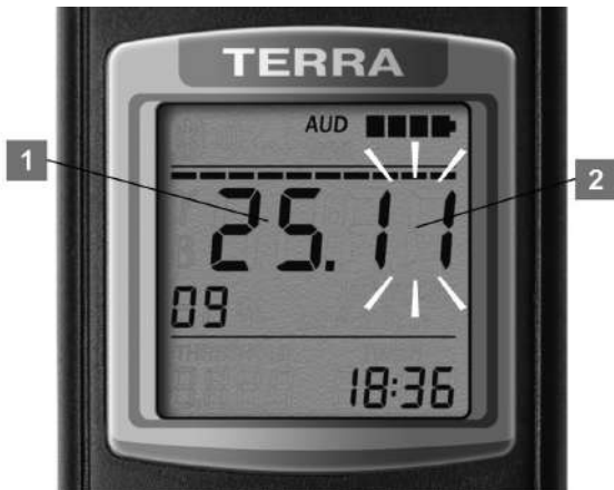
Figure 24 – LCD of the dosimeter (the submode of time and date correction – date programming)
